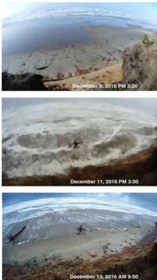
Figure 4.3 Short-term changes in beach morphology captured by a fixed-point webcam, following a storm event. Image reproduced under a Creative Commons Licence © Kako et al. (2018).
