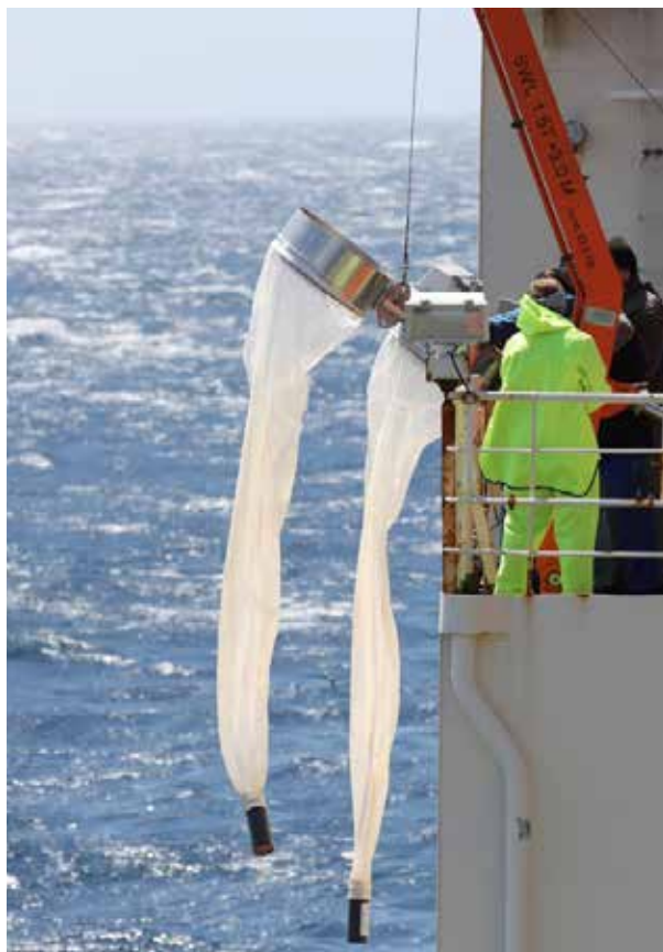
Figure 5.5 The Bongo net captures sub-surface microplastics.
